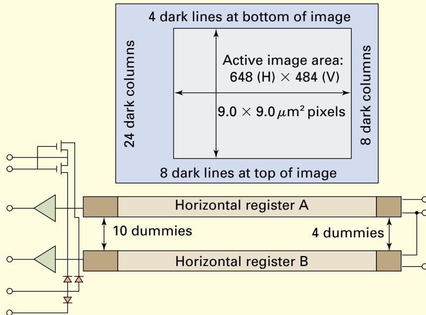
**The Kodak KAI-0330D CCD image sensor uses two horizontal shift registers, each with its own output, to hit 120 frames/sec. A fast-dump feature permits quick dumping of unwanted rows to hit even higher frame rates for reading out a subsection of the full image. This feature lets the chip deliver two full-length rows at 400 frames/sec.**
